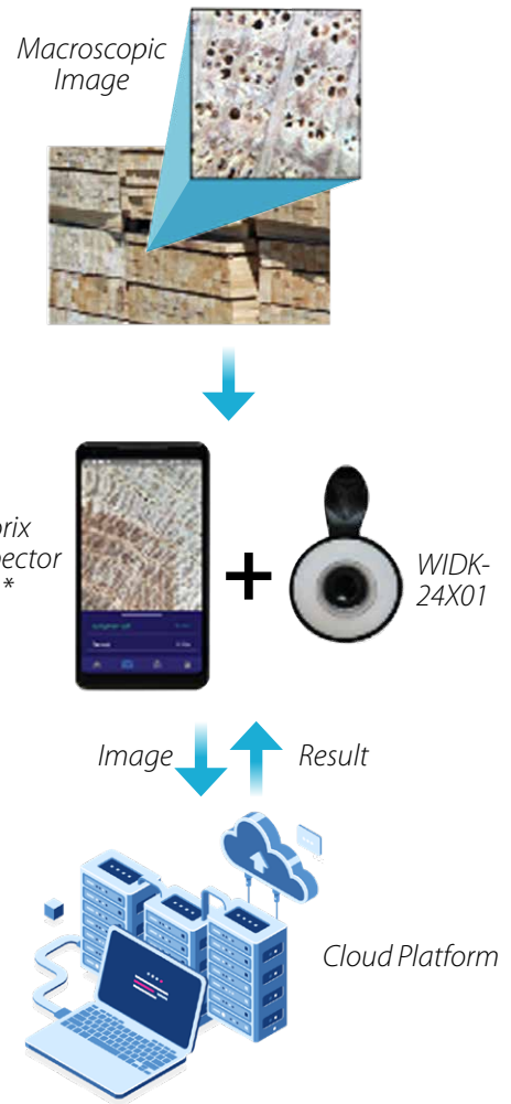
Figure 5: Mobile AI solution for wood identification by Xylorix, Malaysia
