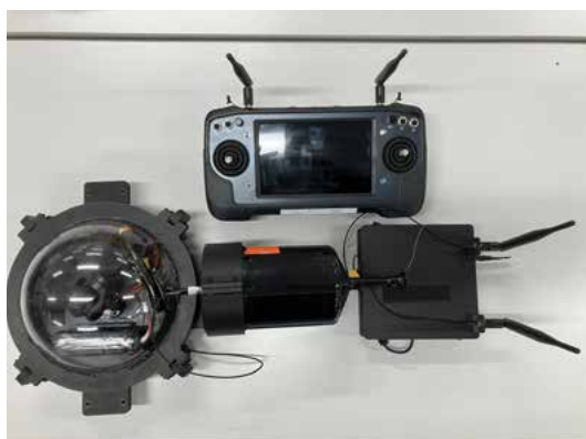
Figure 3: Optical fiber camera system
