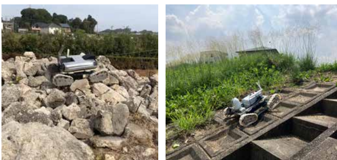
Figure 10: Navigation over debris and slopes
