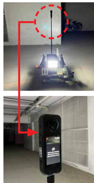
Figure 11: Crawler robot with 360-degree camera and LED
