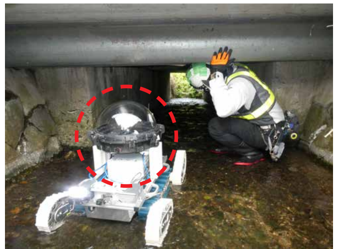
Figure 13: Crawler robot equipped with a gimbal camera
