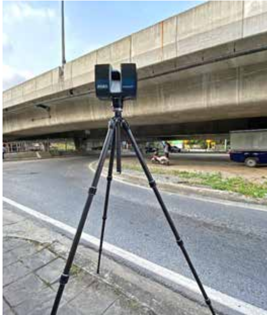
Figure 3: Terrestrial LiDAR Scanner on tripod installation.
