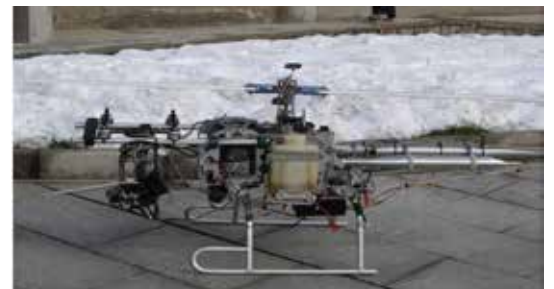
Figure 2 Remotely controlled, pilotless small helicopters with still and video cameras used by the Chinese Search and Rescue Teams for surveying disaster affected areas where access is difficult (National Search and Rescue Training Center, Beijing, China)
