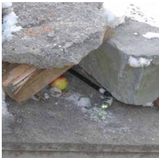
Figure 3 Modern day technology: Cabled sound and light probes used by search and rescue teams today for tracing victims under the debris of a fallen structure.
