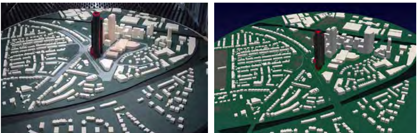
Figure 1: Physical wind tunnel model (left) and CAD model used in the CFD simulations (right).
