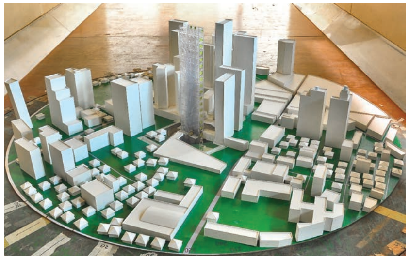
Figure 1: Example of complex surroundings (taken from AIT-TU wind tunnel)
